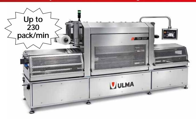
The innovative CMC software (Continuous Motion Control) optimizes the production through an accurate tray positioning control, capable of speeds up to 230 trays/min depending on the type and dimensions of the tray.
